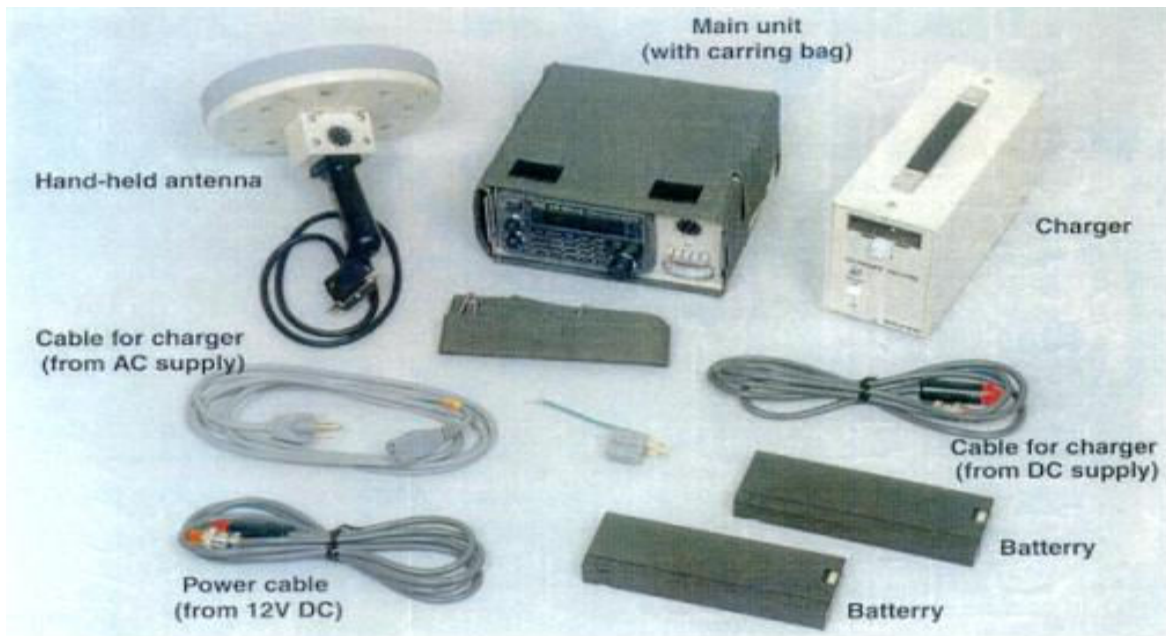
Figure 1 - TD-L8630 Hand Held Radio Direction Finder
